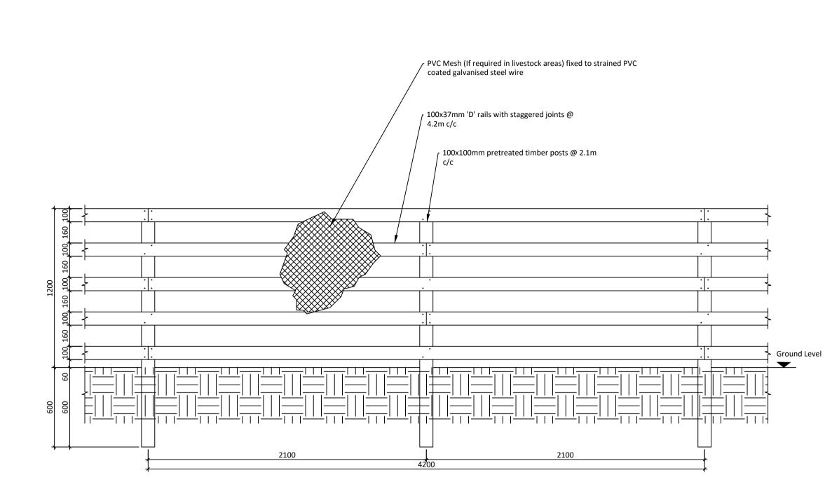
TIMBER POST & RAIL FENCING - ELEVATION VIEW
