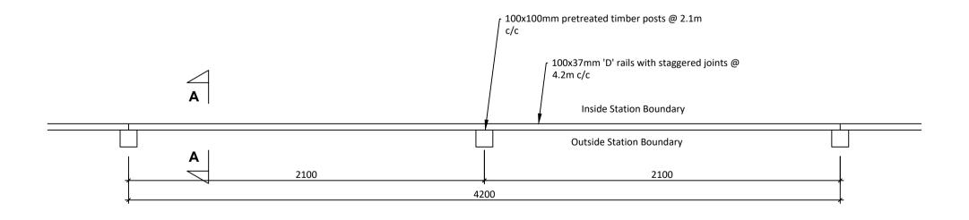
TIMBER POST & RAIL FENCING - PLAN VIEW
